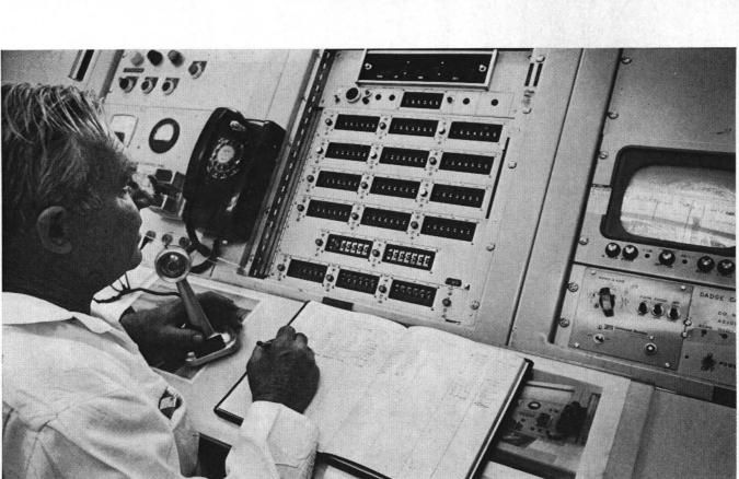
COUNTDOWN SYSTEM at sled track measures not only pre- and post-event time (large readout at top) but also event time for up to 17 different functions with millisecond accuracy. Reid Arrington (7344) is at console.
